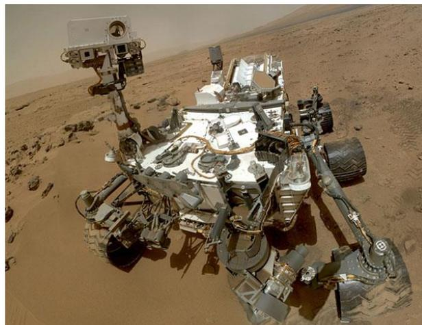
The Mars Curiosity Rover relies on plutonium-238 for power. (Photo credit - NASA)
